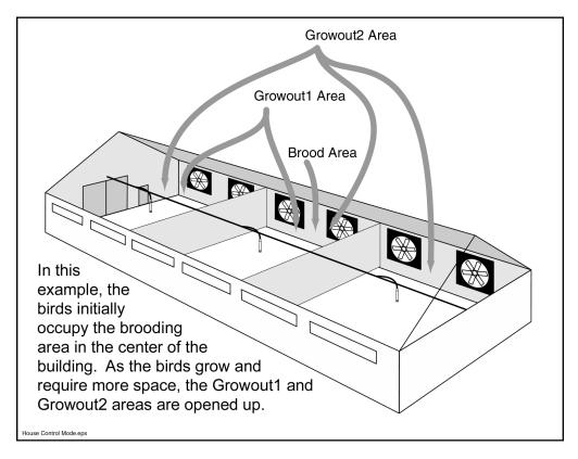
When the House Control Mode is Brood, only sensors in the Brood area are used by the controller.
