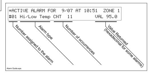
"Zone 0" alarms occur when an alarm relates to all zones (if applicable). For example, a possible hardware problem would generate a Zone 0 alarm.
