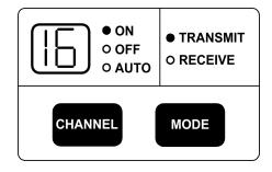
Press the Channel key to select one of the available output channels. Press the Mode key to change the channel's status.
