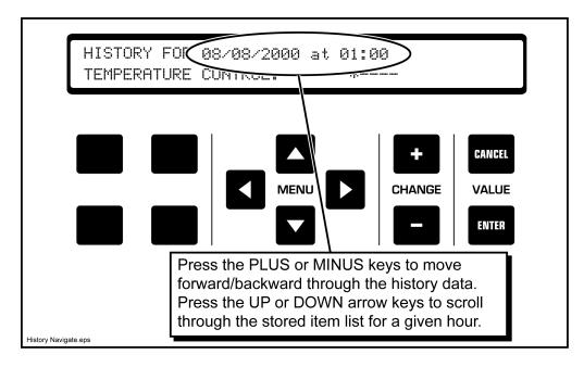
History storage capacity depends on the number of devices that are installed. When the memory storage is almost full, the oldest records are overwritten to make room for the new history.
