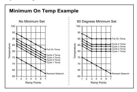
The device will not turn on unless the temperature is at or above the temperature you input here.
