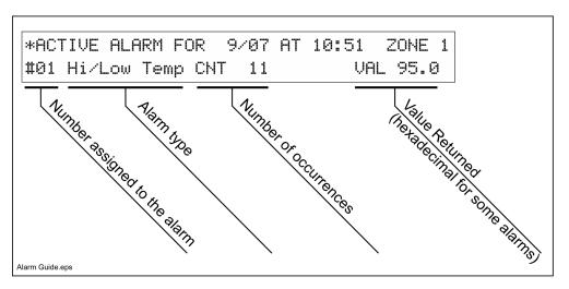
"Zone 0" alarms occur when an alarm relates to all zones (if applicable). For example, a possible hardware problem would generate a Zone 0 alarm.
