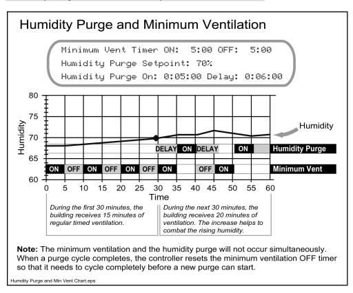
We suggest setting the Humidity Purge Delay slightly longer than the minimum ventilation cycle. The Humidity Purge ON time should be similar to the Minimum Vent Timer ON. This approach increases the amount of ventilation the building receives as humidity increases.
