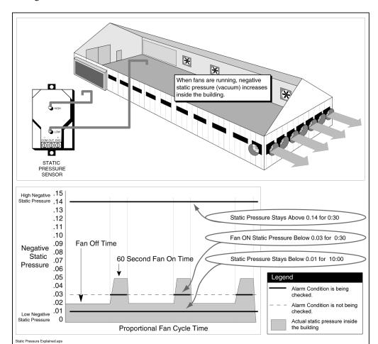
The following illustration provides an example of the possible static pressure alarm settings.
