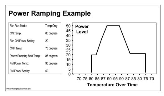
Observe that fan power stays at zero until the ON Temp is reached. As temperature falls the power stays at the Fan ON Power setting until the OFF Temp is reached.
