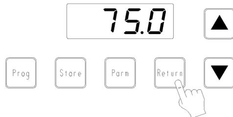
**NOTE:** If the TVS is left displaying a parameter it will revert back to normal operation in 1 minute automatically. If **STORE** was not pressed the displayed parameter will change back to its previous value.
