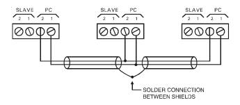
Line-up the comlink card with the connector and insert it in the upright position (see illustration beside). For communication, always use a 1 twisted pair shielded cable. The maximum length of the cable is 3000m and the recommended wire diameter is 1.0 mm. Use a lightning protection module when running the cable between buildings.
