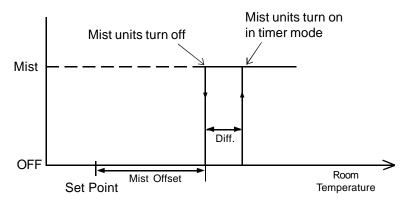
If the humidity compensation is activated, the mist units are turned off when the humidity reaches a user-defined maximum humidity level.
