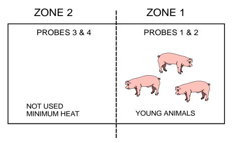
great and zone 1 fans operate according to the average temperature for both zones, cooling in zone 1 may be insufficient. A built-in protection will operate the fans according to the probes of the zone with the highest temperature whenever the temperature difference between zones is greater than a user-defined value.
