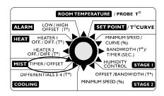
Using the adjustment knob, set the differential to the desired value.
