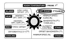
The temperature set point is the target room temperature. It can be adjusted between -40.0°F and 99.9°F (-40.0°C and 37.7°C).
