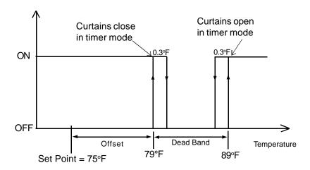
In the example above, when the temperature rises to 89° F, the curtains begin to open and continue to do so until fully open if the temperature remains above this point. If the temperature falls to 88.7° F, the curtains stop opening.
