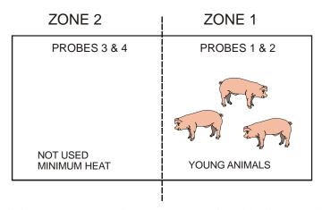
Both heating zones can have negative and positive heater offsets. Using a negative offset allows activating the heating output above the temperature set point; this can be useful to control heat mats for instance.
