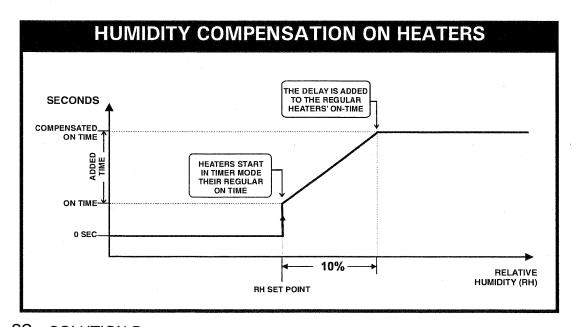
creases proportionally to compensate for the change. The heaters reach their full On-Time when the humidity is at or above RH Set Point + 10% as shown below. Set the dipswitch #6 to ON to use this function.
