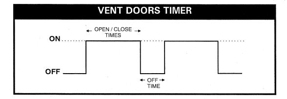
If the pressure has not reached the desired value after the Off Time, the cycle starts again, up until the pressure goes back into the normal range.
