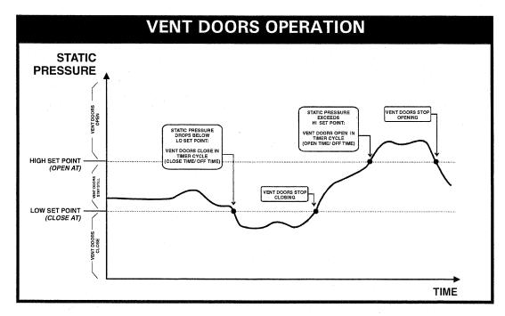
In minimum ventilation, the vent doors open during the pre-opening delay before fans start running. The same delay is used to close the vent doors when the stage 1 fans return to a stop.
