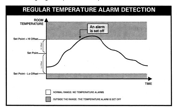
When the average room temperature exceeds the high temperature alarm setting (Set Point + Hi Offset), a high temperature alarm is generated. When the average room temperature drops below the low temperature alarm setting (Set Point - Lo Offset), a low temperature alarm is generated.
