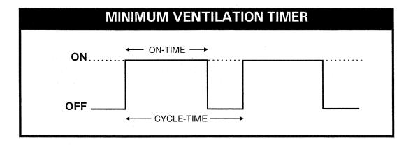
In minimum ventilation cycles, stage 1 fans run according to a timer (On-Time and Cycle Time) as shown above. Either ON/OFF or variable outputs can be used to ensure this type of ventilation.
