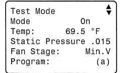
The controller then displays the fan stage that is activated, in accordance with the selected temperature. It also displays the current program in use and the static pressure readings (if a static pressure sensor is used). These values are displayed as readings, they cannot be modified.
