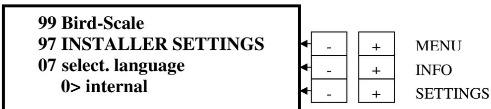
Press **INFO “+”** to go to **line 07**. This is preset to **Internal** for use with a single BE-SSC-101 installation. If a multiple BE-SSC-101 installation is used, then press the **SETTINGS “+”** button to change to **External**.
