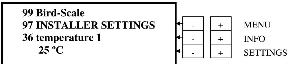
Press **INFO “+”** to go to **line 36**. If the temperature sensor is connected, the actual temperature will show in either **Celsius** or **Fahrenheit** according to what you’ve input previously. If it shows +100 °C or +212 °F, then the sensors are not connected properly. Check the wire connections.
