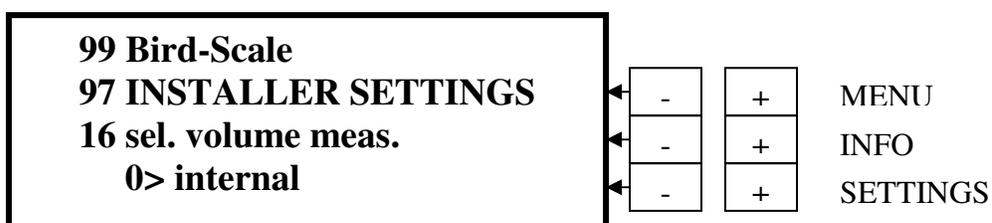
Press **INFO “+”** to go to **line 16**. This is preset to **Internal** for use with a single BE-SSC-101 installation. If a multiple BE-SSC-101 installation is used, then press the **SETTINGS “+”** button to change to **External**.
