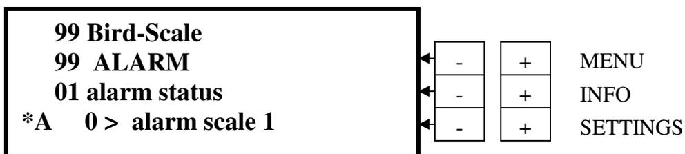
If the system goes into a state of alarm, you'll see the top line **“99 BE-SSC-101 Bird-Scale”** and at the bottom line an **“\*A”**, flashing off & on. There will be an alarm message in **line 0> - e.g. alarm scale 1**
