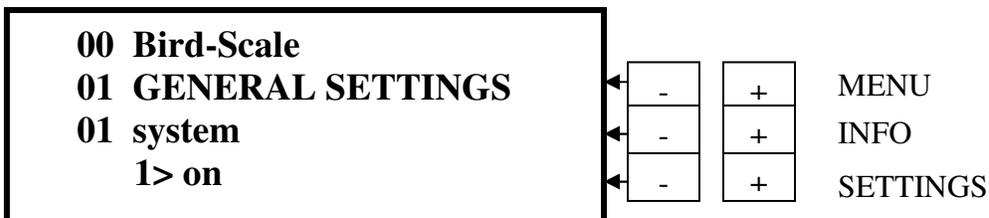
When the Sentinel Scale is installed and first turned on, it will look like this. By pressing the **SETTINGS** “- or +” button will turn the system off or on.
