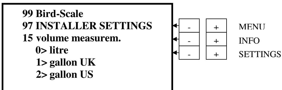
Press **INFO “+”** to go to **line 15**. This is preset to **Litre**. To change the volume measurement from litres to **gallon UK** press **SETTINGS “+”**. To change to **Gallon US** press **SETTINGS “+”** once more.
