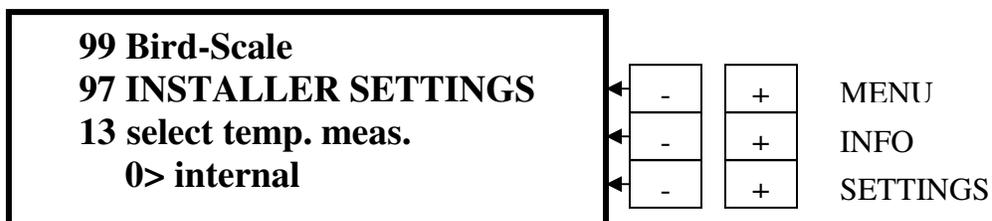
Press **INFO “+”** to go to **line 13**. This is preset to **Internal** for use with a single BE-SSC-101 installation. If a multiple BE-SSC-101 installation is used, then press the **SETTINGS “+”** button to change to **External**.
