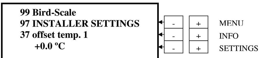
Press **INFO “+”** to go to **line 37**. You can adjust the temperature sensor by pressing **SETTINGS “+ or -”** or if more than one temperature sensor is activated, repeat the above steps for **Lines 38 – 46**. **Normally no action is required here.**
