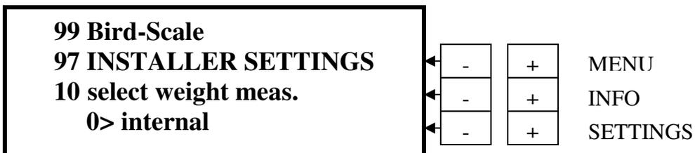
Press **INFO “+”** to go to **line 10**. This is preset to **Internal** for use with a single BE-SSC-101 installation. If a multiple BE-SSC-101 installation is used, then press the **SETTINGS “+”** button to change to **External**.
