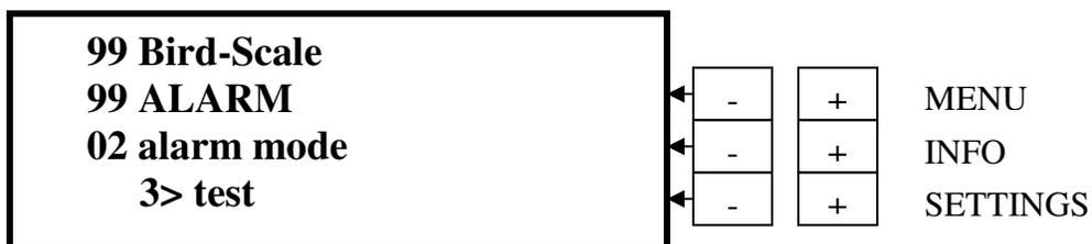
To test the alarm, press **SETTINGS “+”** to get **3> test**. You’ll see the top line **“99 BE-SSC-101 Bird-Scale”** and at the bottom line a **“\*A”**, both will flash on & off. Press **SETTINGS “-”** to go back to **2> on**
