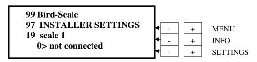
Press **INFO** "+" to go to **info 19.** To connect the scale, press **SETTINGS** "+" to get **1> connected.**
