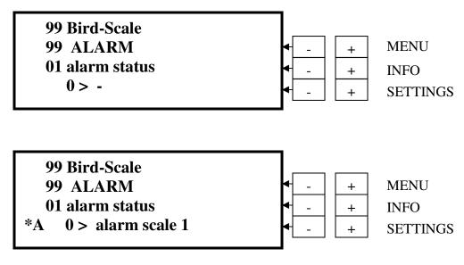
If the system goes into a state of alarm, you'll see the top info **"99 BE-SSC-101 Bird-Scale"** and at the bottom info an **"\*A"**, flashing off & on. There will be an alarm message in **info 0> - e.g. alarm scale 1**
