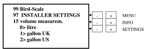
Press **INFO** "+" to go to **info 15.** This is preset to **Litre.** To change the volume measurement from litres to **gallon UK** press **SETTINGS** "+". To change to **Gallon US** press **SETTINGS** "+" once more.
