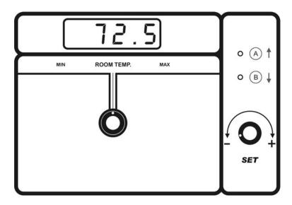
Press push-button A or B until the screen displays "Pr#" (Probe # [number]). If the probe connected to the corresponding terminal <u>is not</u> defective, the screen displays "Pr#" alternating with the temperature measured by the corresponding probe. Otherwise, the letter displays "Pr#" alternating with "Pr#Lo" or "Pr#Hi".
