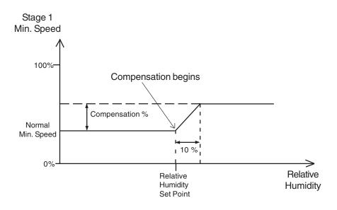
This feature also applies when the minimum ventilation speed is activated. Note that for the compensation to take place, the compensation feature must be activated by the user. When a compensation is applied to the minimum speed, the compensation pilot light turns on.
