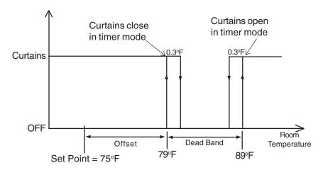
In the example above, when the temperature rises to 89°F, the curtains begin to open and continue to do so until fully open if the temperature remains above this point. If the temperature falls to 88.7°F, the curtains stop opening.
