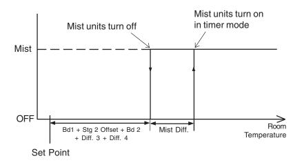
If the humidity compensation is activated, the mist units are turned off when the humidity reaches a user-defined maximum humidity level.
