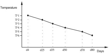
A curve is defined using six points. Each point specifies a day number and a set point for that day. Once the points of the curve are defined, the curve must be activated. The controller will change the temperature set point every hour in a linear fashion between consecutive points of the curve. When the last point of the curve is reached, the temperature set point for that day is maintained until the curve is reactivated.
