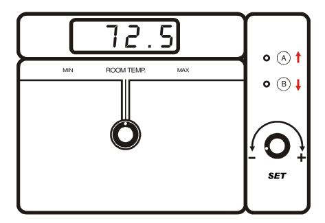
Press push-button A or B until the screen displays "Pr#" (Probe # [number]). If the probe connected to the corresponding terminal is not defective, the screen displays "Pr#" alternating with the temperature measured by the corresponding probe. Otherwise, the letter displays "Pr#" alternating with "Pr#Lo" or "Pr#Hi".
