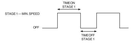
During time on, the Stage 1 fans run at Stage 1 minimum speed. The Stage 1 Pilot Light turns on. During time off, the Stage 1 fans do not run. The Stage 1 Pilot Light turns off. The Stage 1 minimum speed can also be defined by a speed curve (see below).
