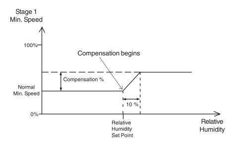
This feature also applies when the minimum ventilation speed is activated. Note that for the compensation to take place, the compensation feature must be activated by the user. When a compensation is applied to the minimum speed, the compensation pilot light turns on.
