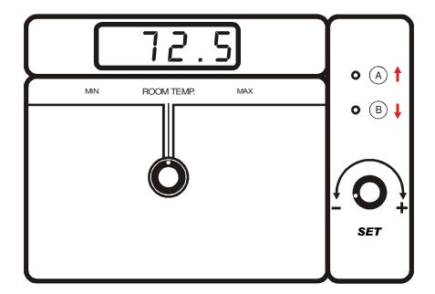
Press push-button A or B until the screen displays "Pr#" (Probe # [number]). If the probe connected to the corresponding terminal <u>is not</u> defective, the screen displays "Pr#" alternating with the temperature measured by the corresponding probe. Otherwise, the letter displays "Pr#" alternating with "Pr#Lo" or "Pr#Hi".
