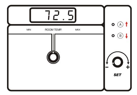
Press push-button A or B until the screen displays "Pr#" (Probe # [number]). If the probe connected to the corresponding terminal is not defective, the screen displays "Pr#" alternating with the temperature measured by the corresponding probe. Otherwise, the letter displays "Pr#" alternating with "Pr#Lo" or "Pr#Hi".
