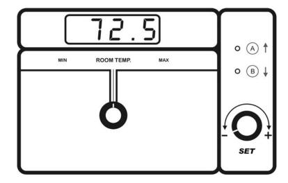
Press push-button A or B until the screen displays "**Pr#**" (Probe # [number]). If the probe connected to the corresponding terminal <u>is not</u> defective, the screen displays "**Pr#**" alternating with the temperature measured by the corresponding probe. Otherwise, the letter displays "**Pr#**" alternating with "**Pr#Lo**" or "**Pr#Hi**".
