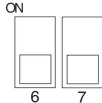
Note that if only one stage is used for heating, it must be Stage 6.
