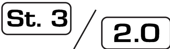
(ii) If, after about 6 seconds, no action is taken by the user, the absolute temperature value is displayed, alternating with "St. 3". In this case, the absolute value is: Set Point + Bandwidth 1 + Offset 2 + Bandwidth 2 + Differential 3.
