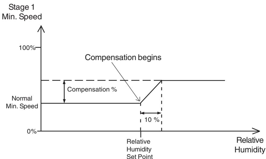
This feature also applies when the minimum ventilation speed curve is activated. Note that for the compensation to take place, the compensation feature must be activated by the user. When a compensation is applied to the minimum speed, the compensation pilot light turns on.
