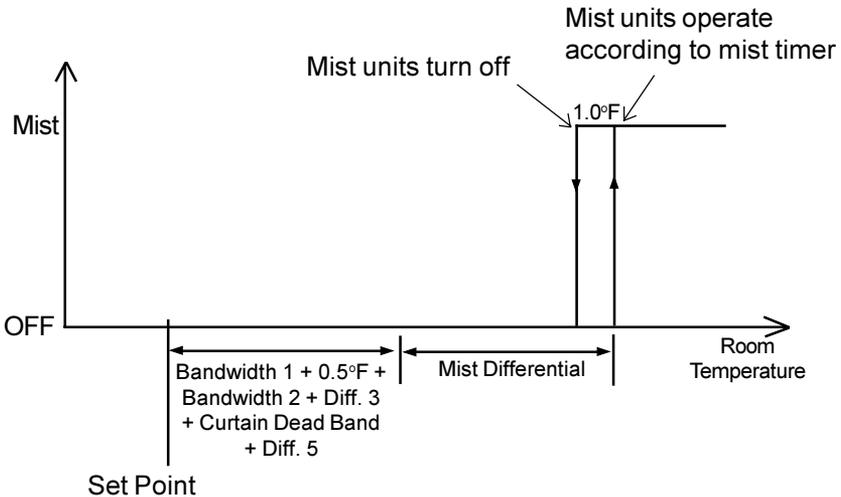
The mist units operate according to the mist time on and time off settings:
