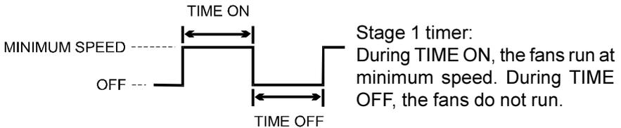
The fans can be set to operate in three different ways:
