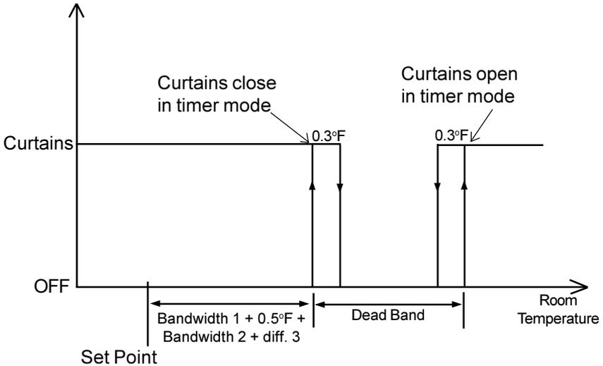
The curtains open and close intermittently according to the time on and time off settings:
