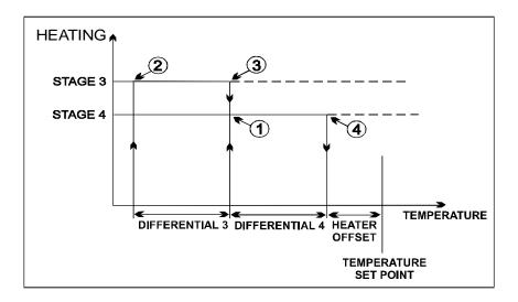
When stages 3 and 4 are used for heating, stages 1 and 2 operate as described for cooling. Stages 3 and 4 operate as described hereafter.
