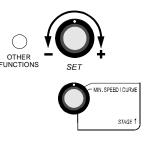
The single minimum speed can be adjusted even if the minimum speed curve is activated as long as it is not effectively in operation. If the curve is in operation, deactivate the curve as described below.
