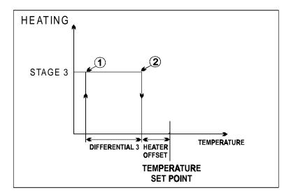
When stage 3 is used for heating, stages 1 and 2 operate as described for cooling. However stage 3 operates at room temperatures below the set point, as described hereafter.
