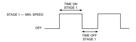
Time on [seconds] - When the stage 1 fans operate according to the minimum ventilation cycle, they run during time on.
