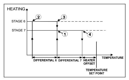
When stages 6 and 7 are used for heating, stages 1, 2, 3, 4 and 5 operate as described for cooling. However stages 6 and 7 operate at room temperatures below the set point, as described hereafter.
