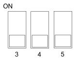
FACTORY SETTING: When the controller is shipped from the factory, switches # 3, 4 and 5 are set to OFF (probes are deactivated).
