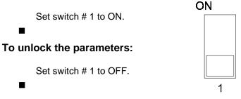
FACTORY SETTING: When the controller is shipped from the factory, switch # 1 is set to OFF (the parameters are unlocked).
