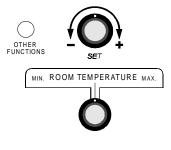
The room temperature shown on the display is the average value of all temperatures measured by probes that are activated and in proper operating condition.
