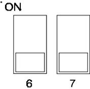
**FACTORY SETTING:** When the controller is shipped from the factory, switch # 6 and 7 are set to OFF (stages 3 and 4 used for cooling).
