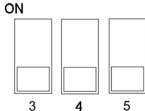
**FACTORY SETTING:** When the controller is shipped from the factory, switches # 3, 4 and 5 are set to OFF (the probes are deactivated).
