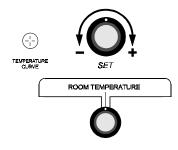
■ Press the push-button. The word "PR1" and the temperature measured by the probe connected to terminal # 1 (supplied with the controller) alternately appear on the display.
