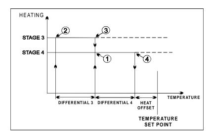
When stages 3 and 4 are used for heating, stages 1 and 2 operate as described for cooling. However stages 3 and 4 operate at room temperatures below the set point, as described hereafter.
