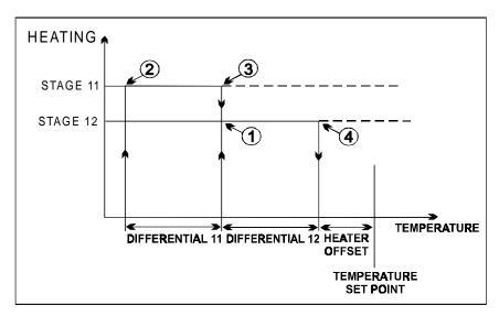
When stages 11 and 12 are used for heating, stages 1 through 10 operate as described for cooling. However stages 11 and 12 operate at room temperatures below the set point, as described hereafter.
