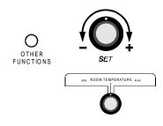
■ Press the push-button. The word "PR1" and the temperature measured by the probe connected to terminal # 1 (supplied with the controller) alternately appear on the display.
