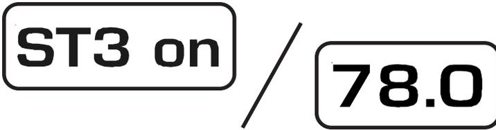
(iii) When the user turns the adjustment knob to make an adjustment to the stage 3 differential, the relative value reappears on the display.
