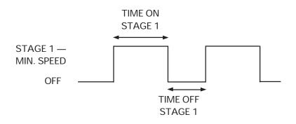
During the Time On, stage 1 fans run at their minimum speed and the pilot light of stage 1 is lit; during the Time Off, the fans return to a stop and the pilot light turns off. Note that the minimum speed of stage 1 can automatically be adjusted over time with a ramp (see below).
