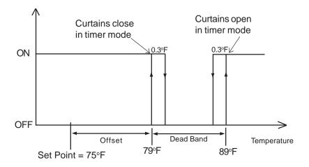
In the example above, when the temperature rises to  $89^{\circ}$ F, the curtains begin to open and continue to do so until fully open if the temperature remains above this point. If the temperature falls to  $88.7^{\circ}$ F, the curtains stop opening.
