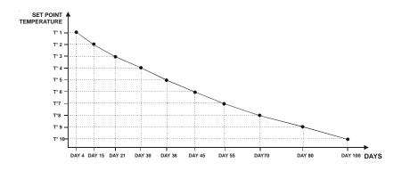
A ramp is defined using ten points. Each point specifies a day number and a set point for that day. Once the points of the ramp are defined, the ramp must be activated. The controller will change the temperature set point every hour in a linear fashion between consecutive points of the ramp. When the last point of the ramp is reached, the temperature set point for that day is maintained until the ramp is reactivated.
