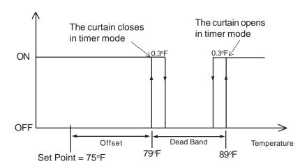
In the example above, when the temperature rises to 89°F, the curtain starts opening and continues to do so until fully open if the temperature remains above this point. If the temperature falls to 88.7°F, the curtain stops opening.
