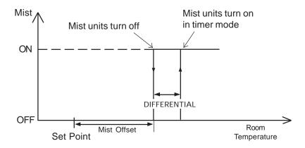
Mist units start running according to a timer cycle (Time On and Time Off) when their start temperature is reached (Set Point + Mist Offset + Differential).
