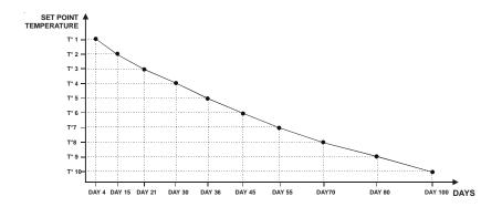
A ramp is defined using ten points. Each point specifies a day number and a set point for that day. Once the points of the ramp are defined, the ramp must be activated. The controller will change the temperature set point every hour in a linear fashion between consecutive points of the ramp. When the last point of the ramp is reached, the temperature set point for that day is maintained until the ramp is reactivated.
