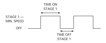
During the Time On, stage 1 fans run at their minimum speed and the pilot light of stage 1 is lit; during the Time Off, the fans return to a stop and the pilot light turns off. Note that the minimum speed of stage 1 can automatically be adjusted over time with a ramp (see below).
