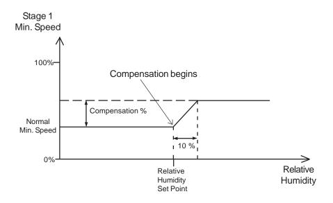
When a compensation is applied to the minimum speed, the compensation pilot light turns on.
