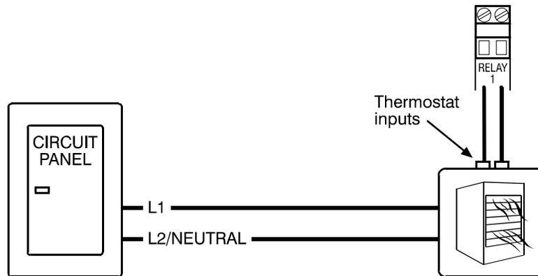
**PB-1/3: gas furnace or brooder – power connections**
