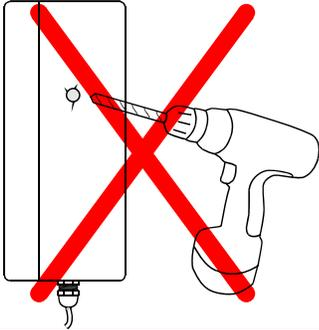
Use the electrical knockouts for bringing wires or cables into or out of the enclosures. Use watertight strain reliefs or conduit connectors at all cable-entry points.
