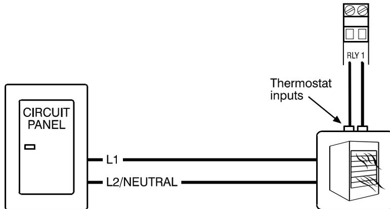
**PB-2/4/5: gas furnace or brooder – power connections**
