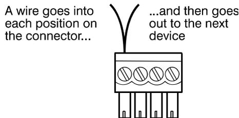
The last device on a communication channel must have the termination resistors in place or a termination module installed. For the location of the termination resistors on Power Blocks, see **Microboard layout** on page 34. For other OMNI devices, see the installation guide for the particular device.
