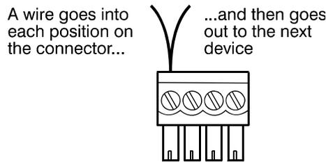
The last device on a communication channel must have the termination resistors in place or a termination module installed. For the location of the termination resistors, see the device’s installation guide.
