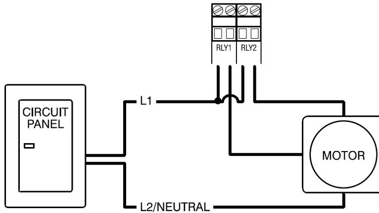
**Connecting single-stage heating or cooling elements**
