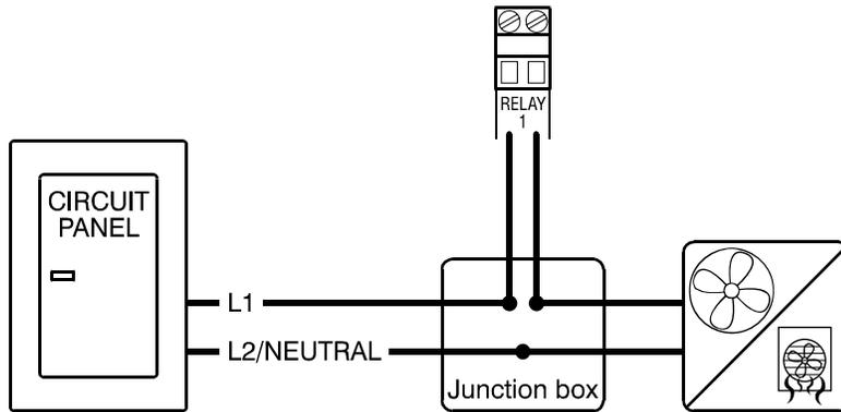
**PB-2/4/5: gas furnace or brooder – thermostat inputs**
