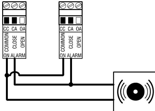
**Normally closed system (open on alarm)**
