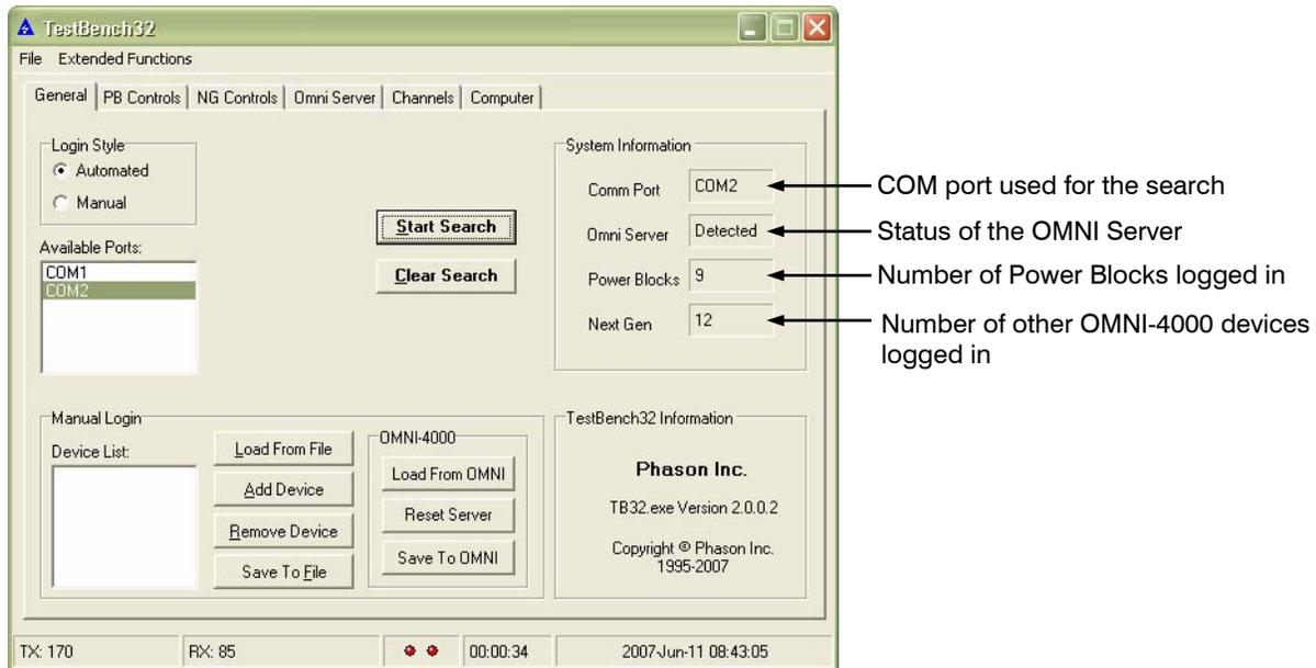
4. Under *Available Ports*, select the communication port that has the OMNI Server connected.
