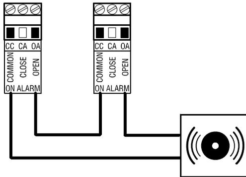
**To connect an alarm system to a PB-2/4/5**
