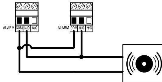
**Normally closed system (open on alarm)**
