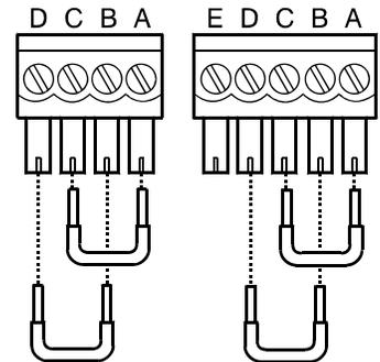
Loopback tests help verify the integrity of the communication line. During the tests, the computer sends out information along the communication cable. The information “bounces back” when it gets to the loopback connector. The computer compares the information it receives back; if it is the same as the information sent out, then both the send (TX) and receive (RX) lines are intact.
