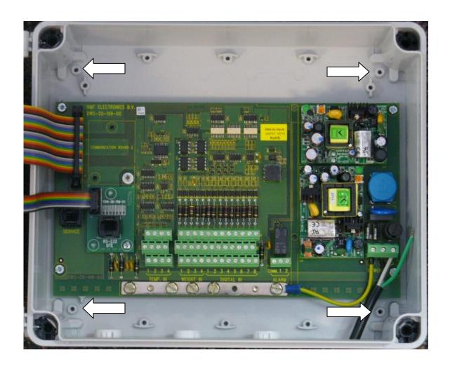
Using the 4x mounting screws located inside the bag containing the strain relief nuts, mount the controller in 4x locations shown by arrows in pictorial above.
