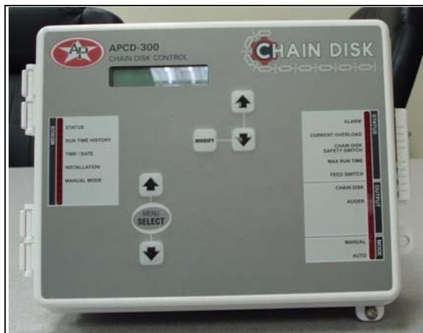
Fig. 10-D Chain Disk Control Unit APCD-300
