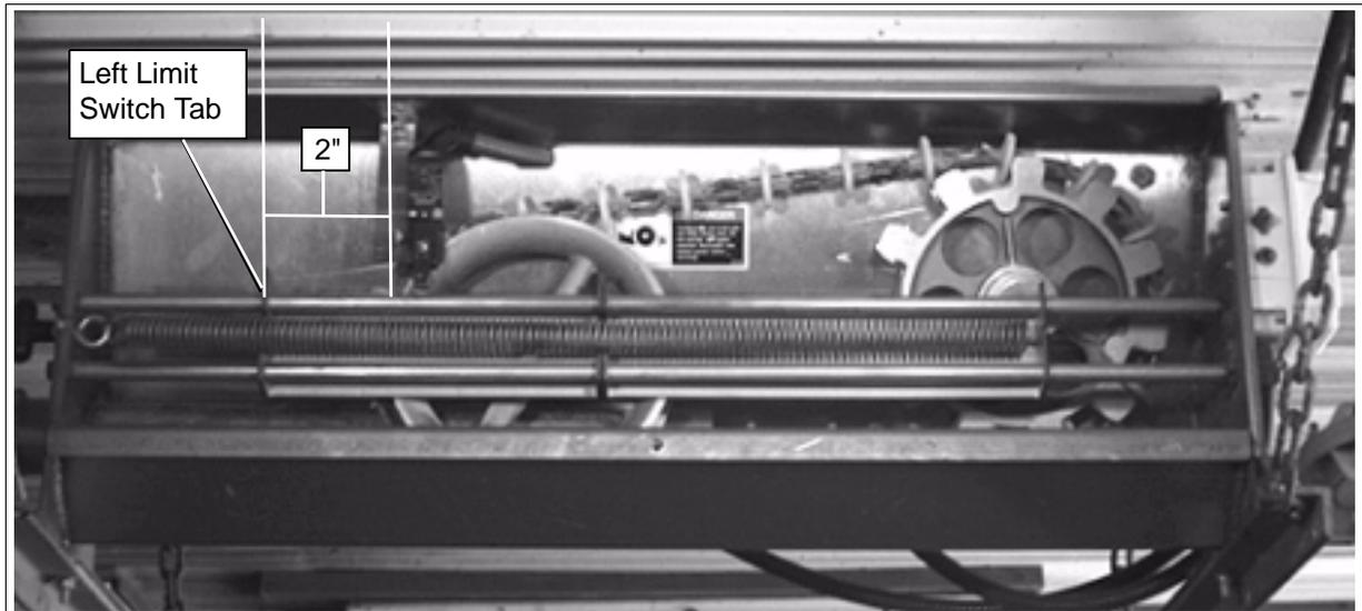
**Figure 16C** *Limit Switch Adjustment*
