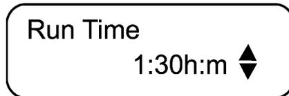
3. Press MODIFY then use the arrow keys to set this parameter to the desired value. Press MODIFY once again to validate.
