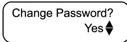
1. Press MODIFY. The first two digits of the password flash on the display.
