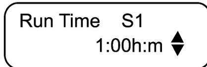
5. Press MODIFY then use the arrow keys to set this parameter to the desired value. Press MODIFY once again to validate.
