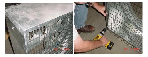
Step 12. Install either another guard screen or a shutter on the exhaust side of the fan. To install another guard screen repeat Step 10. To install an exhaust shutter refer to the installation instructions IS10024 that come with the shutter kit.
