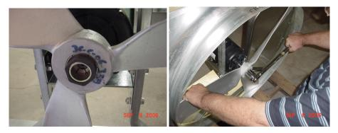
Step 9. Once the blade has been installed, rotate the blade and check to ensure equal tip clearance all the way around the orifice. Some lateral adjustment of the motor plates may be necessary to achieve blade centering.
