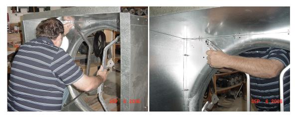
Step 6. Position the motor plates as shown in photo below with the motor plate flush with motor mount tubes Making sure that front edge of the motor plates are parallel with the motor mount tubes (refer to photo below), tighten securely (approximately 15 - 20 ft. lbs.).
