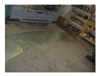
Step B Form the flat cone sections into a cone by joining flange #1 and flange #8 and using three  $\frac{1}{4}$ "-20 x  $\frac{3}{4}$ " bolts (# MH8061) and nuts (# MH8055), bolt the two flanges together. Again make sure that the lapping of panels is the same as all other cone seams. As in Step #A install the bolt closest to the narrow end of the cone and apply a cone support strap to the outside of the cone panels.
