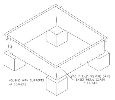
Step 4. Insert the orifice into the box so the throat is farthest away from the box flange. Loosely fasten the orifice to the box using  $\frac{1}{4}$ " - 20 X  $\frac{3}{4}$ " bolts and nyloc nuts. Insert the bolts from the outside, inward. Complete the fastening of the box together using #10 x  $\frac{1}{2}$ " sq. drive sheet metal screws. Now you can tighten all the  $\frac{1}{4}$ " – 20 X  $\frac{3}{4}$ " nuts and bolts holding the orifice to the box.
