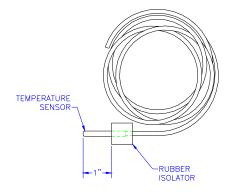
2. Center the rubber isolator (part # SMP90421) into the radiant sensor bracket (part # SMP90940) shield notches as shown in the diagram below and hold in place with the spring hose clamp (part # MH90420).
