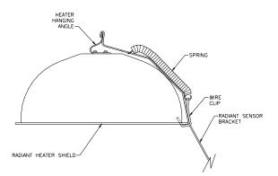
7a.Attach the sensor wire to the radiant heater hanging apparatus ensuring that the sensor wire maintains a minimum clearance of 4" from the heater shield (see drawing below).
