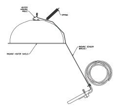
6. Slide the wire clip (part # SMP90941) over the radiant sensor bracket so the short bent ends is to the inside of the bracket. Attach the wire clip (part # SMP90941) to the lower end of the spring (part # ZR1719) and while stretching the spring latch the wire clip over the bottom edge of the heater shield as shown below.
