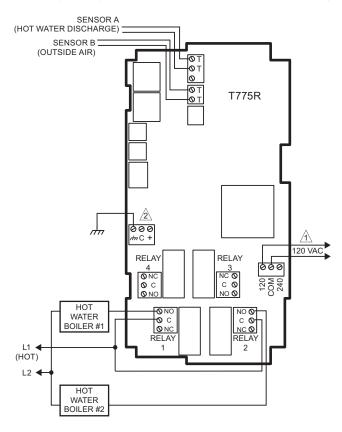
POWER WITH 24 VAC OR 120/240 VAC AT THE APPROPRIATE TERMINAL BLOCK.
