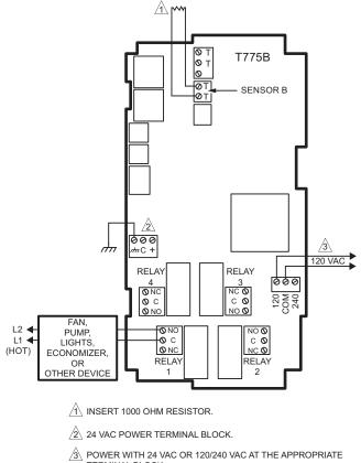
OWER WITH 24 VAC OR 120/240 VAC AT THE APPROPRIATE TERMINAL BLOCK.
