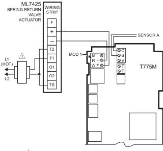
A POWER SUPPLY. PROVIDE DISCONNECT MEANS AND OVERLOAD PROTECTION AS REQUIRED.
