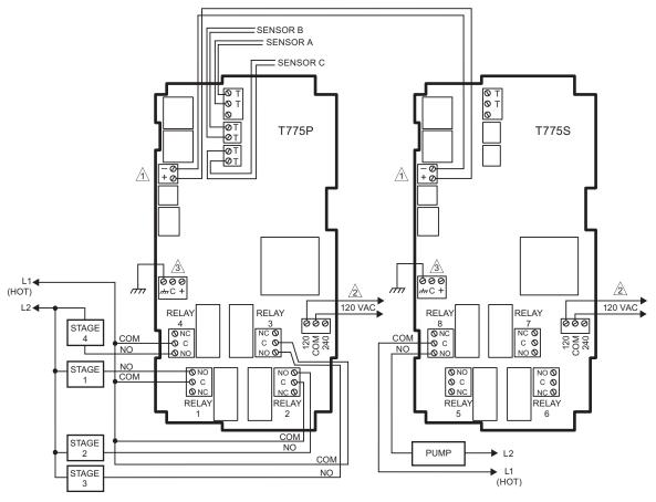
1775 BUS TERMINALS PROVIDE WIRING CONNECTIONS TO/FROM T775P/L AND T775S
