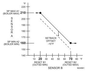
Fig. 2. Reset Curve for First Output with Setback Offset.
