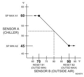
Fig. 15. Chiller Reset Curve.
