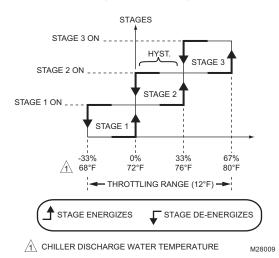
Fig. 23. Chiller Control Staging Behavior (when the effective setpoint = 72° F).
