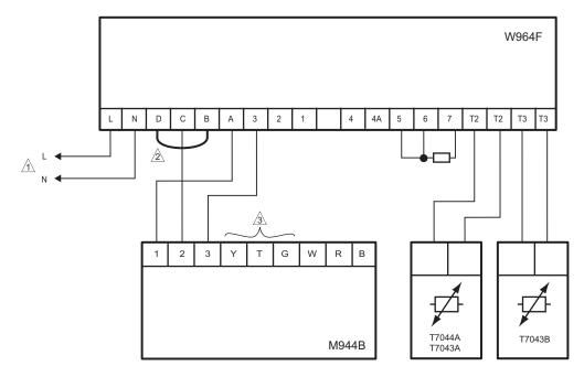
${\underline{\land}}$  120 V, 60 HZ POWER SUPPLY. PROVIDE DISCONNECT MEANS AND OVERLOAD PROTECTION AS REQUIRED.
