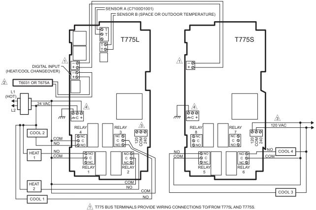
2 SETUP THE CONTROL (T6031 OR T765) SO THAT IT CLOSES ON A TEMPERATURE FALL.
