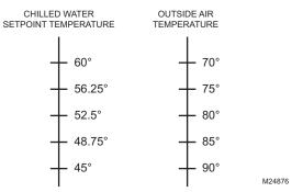
Fig. 17. Chiller Setpoint vs. Outside Temperature.
