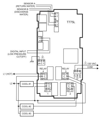
Fig. 29. T775L Wiring - Reciprocating Chiller.
