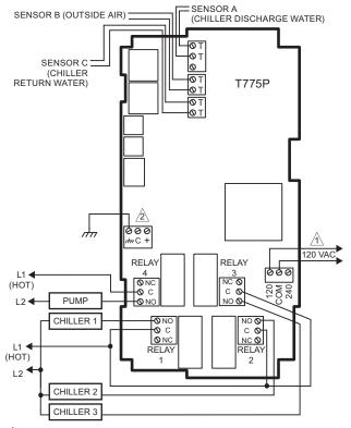
$\underline{\land}$  Power with 24 Vac or 120/240 vac at the appropriate terminal block.
