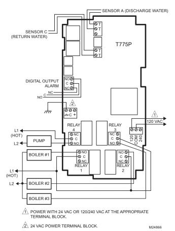
Fig. 19. T775P Wiring - Multi-Stage Boiler Control (No Reset).
