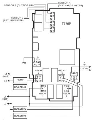
A POWER WITH 24 VAC OR 120/240 VAC AT THE APPROPRIATE TERMINAL BLOCK.
