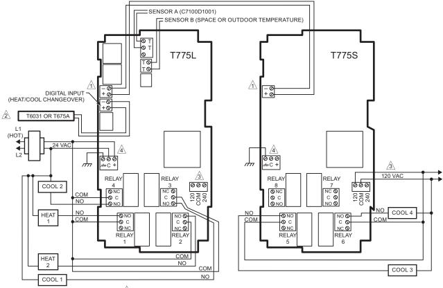
T775 BUS TERMINALS PROVIDE WIRING CONNECTIONS TO/FROM T775L AND T775S.
