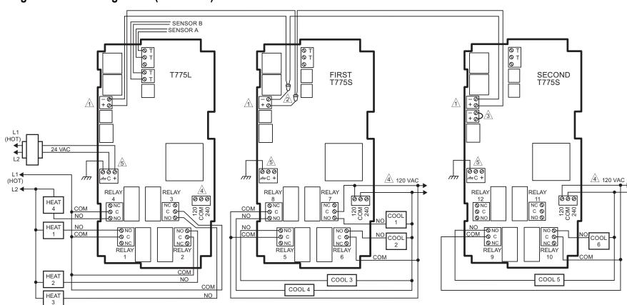
1775 BUS TERMINALS PROVIDE WIRING CONNECTIONS TO/FROM T775L AND T775S.
