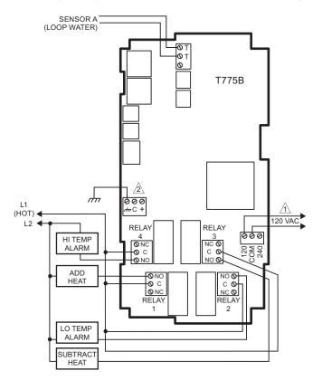
$\triangle$  POWER WITH 24 VAC OR 120/240 VAC AT THE APPROPRIATE TERMINAL BLOCK.
