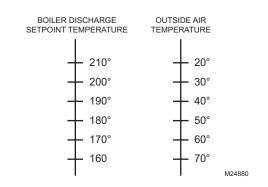
Fig. 28. Boiler Discharge Temperature vs. Outside Temperature.
