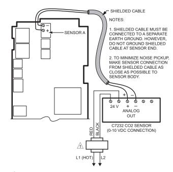
LSE SEPARATE 24 V TRANFORMER TO POWER THE C7232 CO2 SENSOR. PROVIDE DISCONNECT MEANS AND OVERLOAD PROTECTION AS REQUIRED.
