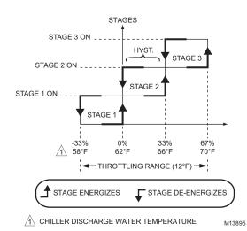
Fig. 30. Chiller Control Staging Behavior (when the effective setpoint = 62° F (17° C)).
