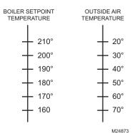
Fig. 14. Boiler Discharge Temperature Setpoint vs. Outside Temperature.
