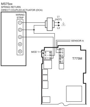
A POWER SUPPLY, PROVIDE DISCONNECT MEANS AND OVERLOAD PROTECTION AS REQUIRED.
