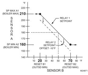
Fig. 10. Hot Water Reset Curve.
