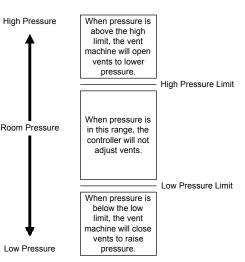
The Photohelic gauge has two knobs on the Dwyer gauge, one for the Low limit and one for the high limit. Turn the knob clockwise to increase the setting and counterclockwise to decrease.
