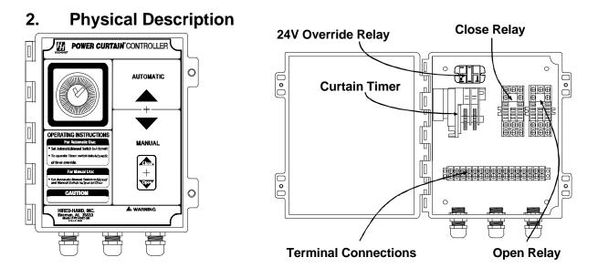
The picture on the left above is the front of the controller. The picture on the right is a picture of the internals of the controller showing major components.
