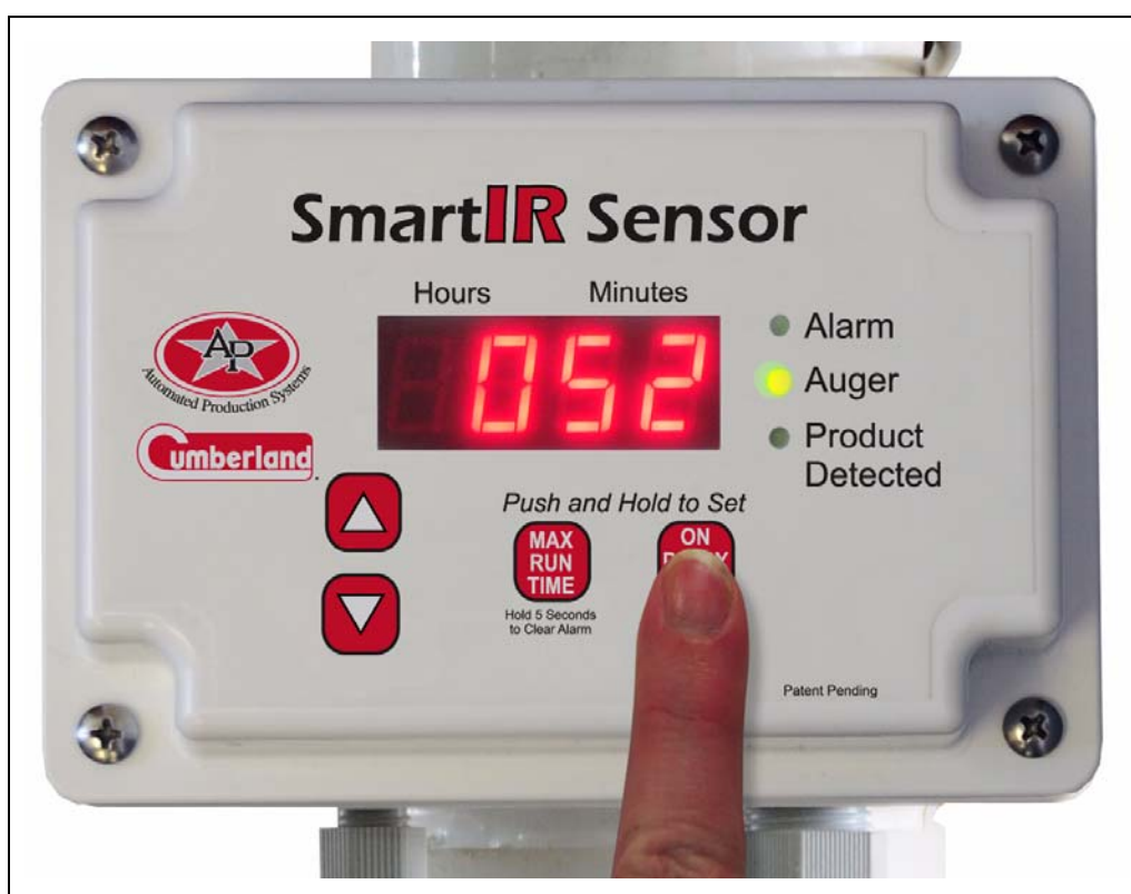
Figure 5A Checking Delay Time
