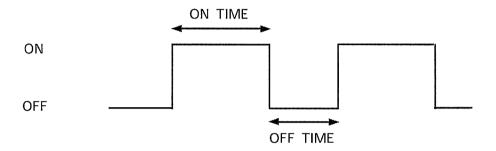
When the cooling cycle starts (**On Temp**), the output is activated using the **minimum ON time**. The ON time gradually increases as the room temperature increases. The **maximum ON time** is reached when the room temperature reaches the output's Max Temperature (**T° Max**). The Off Time never changes. The following graphic illustrates the situation:
