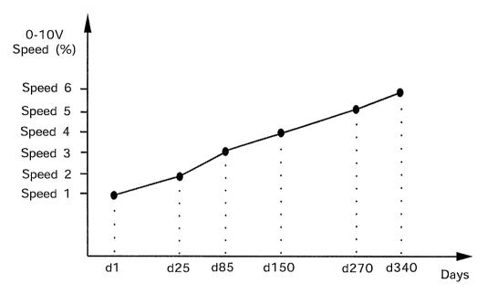
A curve is defined using up to ten points. Each point specifies a day number and a minimum speed for that day. Once the points of the curve are defined, the curve must be activated. The controller will change the minimum speed value every hour in a linear fashion between consecutive points of the curve. When the last point of the curve is reached, the minimum speed for that day is maintained until the curve is reactivated.
