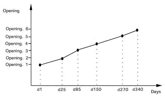
A curve is defined using up to ten points. Each point specifies a day number and a minimum opening for that day. Once the points of the curve are defined, the curve must be activated. The controller will change the minimum opening value every hour in a linear fashion between consecutive points of the curve. When the last point of the curve is reached, the minimum opening for that day is maintained until the curve is reactivated.
