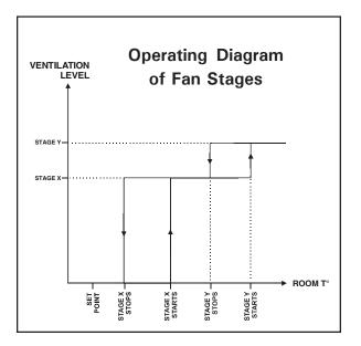
Start temperatures of fan stages are defined with respect to the set point and with respect to each other. This means that when one of these values is adjusted, all the consecutive values are adjusted by the same amount. For example, if the set point is increased by  $1^{\circ}F$ , the start temperature of all fan stages will be increased by the same amount.
