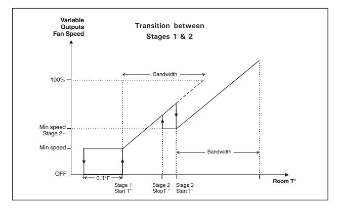
The **bandwidth** is the temperature interval over which variable outputs go from their minimum to their maximum speed. This is true even if full speed is never reached as in the example above: when stage 2 starts, the controller decreases the speed of variable outputs to the initial speed associated with stage 2. It then uses the bandwidth to increase the fan speed as the room temperature rises.
