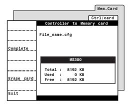
• Once the transfer is over, press Exit then remove the memory card from the connector.
