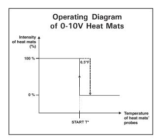
0-10V heat mats starts operating at its full intensity (100%) when the average temperature of chosen sensors reaches the start temperature of the output. It is disabled when the temperature rises  $0.5 \,^{\circ}$ F (0.3  $^{\circ}$ C) above the start temperature.
