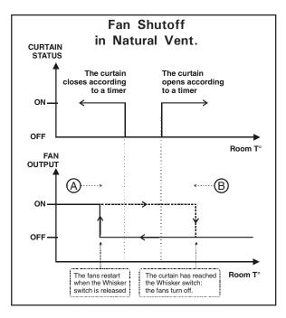
**Security:** If the temperature drops suddenly or if the whisker switch is defective, the controller automatically restarts the fans when the temperature falls  $5^{\circ}F(3^{\circ}C)$  below the lowest curtain's closing temperature. When this situation occurs, a defective whisker switch alarm is posted to the alarm log.
