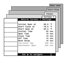
Wind Delay When the controller is in natural ventilation and temperature falls below the "Start Close At" temperature or rises above the "Start Open At" temperature, the curtain only starts moving after the wind delay has elapsed. This way, the curtain does not move when wind drafts cause sudden temperature changes. Set the wind delay to the desired value. Adjustable from 0 to 900 seconds (15 minutes).
