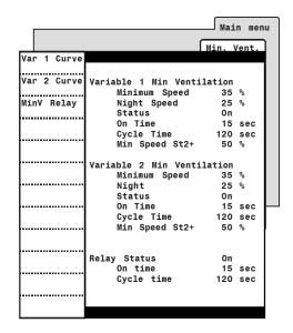
Min Speed Stage 2+ for Var. Outputs 1-2 Set the speed at which each variable output starts running at the beginning of stage 2 and beyond (see sec. 6.2).
