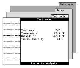
Switch on the test mode status then set the simulated inside & outside temperature and the humidity level.
