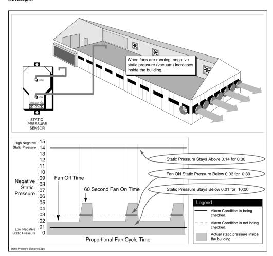
The following illustration provides an example of the possible static pressure alarm settings.
