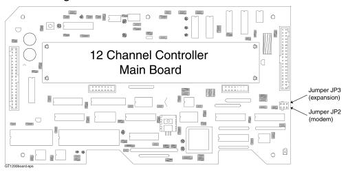
If the **Egg Producer is not** at the terminal end of a group of controllers (all attached to a modem), the **Egg Producer JP2** needs to be changed to not terminated on the "modem" communications line.
