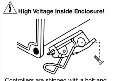
Controllers are shipped with a bolt and nut to hold the quick release latch closed. You can remove the bolt and nut during the installation process. You must replace these after installation to protect against accidental exposure to the high voltage inside the enclosure.
