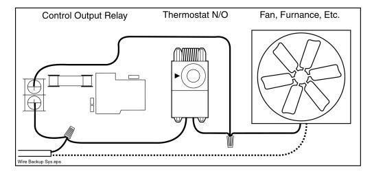
Thermostats should be installed to backup heaters, fans and inlets. Natural ventilation buildings need curtain drops. Thermostats can be wired to the devices they will operate, and in parallel with the controller as shown above.
