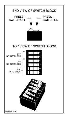
Any odd-numbered channel can be interlocked with the next even-numbered channel (1 & 2, 3 & 4, and so on).
