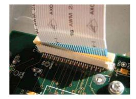
Latch open (FCC cable unlocked)
