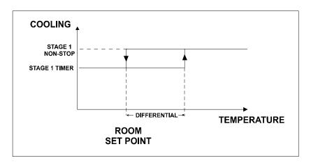
**Temperature Rises:** When the room temperature is below the set point, the Stage 1 fans operate in timer mode to provide minimum ventilation (see below). When the temperature rises above the set point by a value equal to the differential, the Stage 1 fans operate continuously.
