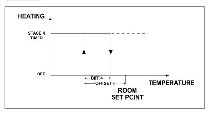
**Temperature Falls:** When the room temperature drops below the set point by a value equal to the offset, the stage 4 heaters operate in timer mode.
