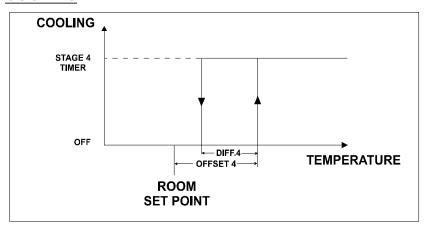
**Temperature Rises:** When the room temperature is below the set point plus the offset, the Stage 4 fans or mist units do not operate. When the temperature rises above the set point by a value equal to the offset, the Stage 4 fans or mist units operate in timer mode (see below).
