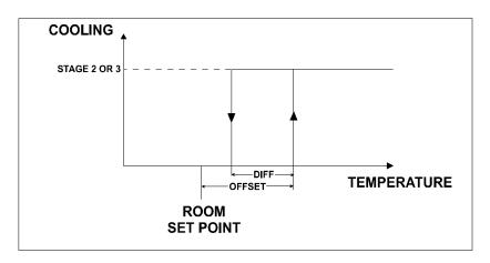
**Temperature Rises:** When the temperature rises above the set point by a value equal to the offset, the Stage 2 or 3 fans operate continuously.
