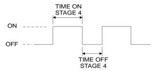
During time on, the Stage 4 fans or heating units are operating. The Stage 4 Pilot Light turns on. During time off, the Stage 4 fans or heating units do not run. The Stage 4 Pilot Light turns off.
