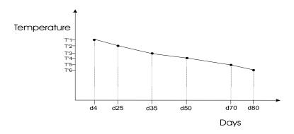
A curve is defined using six points. Each point specifies a day number and a set point for that day. Once the points of the curve are defined, the curve must be activated. The controller will change the temperature set point every hour in a linear fashion between consecutive points of the curve. When the last point of the curve is reached, the temperature set point for that day is maintained until the curve is reactivated.
