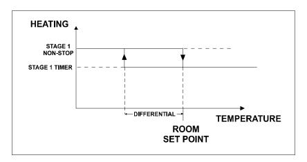
**Temperature Falls:** When the room temperature drops below the set point by a value equal to the differential, the stage 1 heaters stop operating in timer mode and run continuously.
