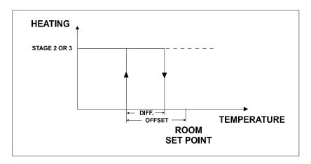
**Temperature Falls:** When the room temperature drops below the set point by a value equal to the offset, the stage 2 or 3 heaters run continuously.
