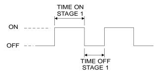
During time on, the Stage 1 fans or heating units are operating. The Stage 1 Pilot Light turns on. During time off, the Stage 1 fans or heating units do not run. The Stage 1 Pilot Light turns off.
