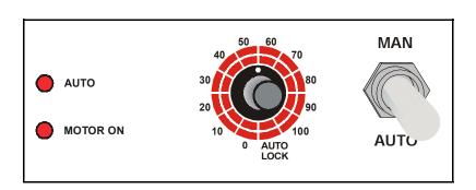
The CIP-1/6 faceplate (shown above) features one toggle switch, one position knob and two status LEDs. The toggle switch is used to select whether the actuator motor operates in auto mode or under manual.
